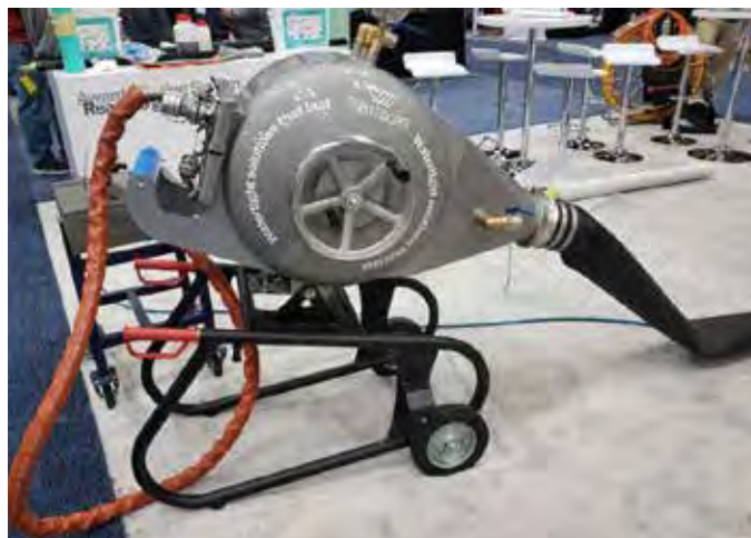
Portable inversion drum
