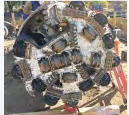
Auger-driven SBU for drilling through rock
