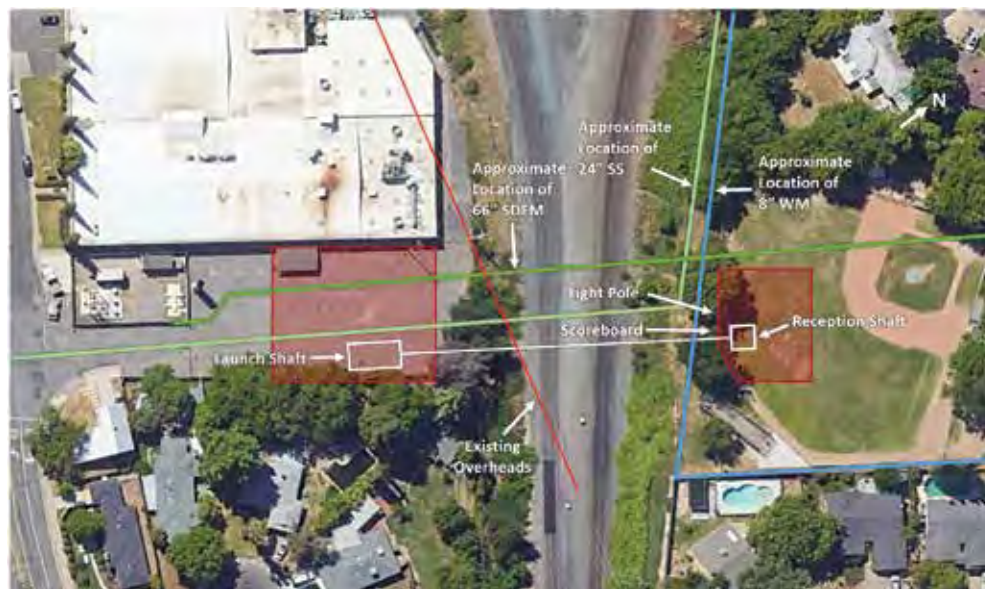
Figure 1. Aerial view of guided boring crossing of the two sets UPRR tracks showing key project constraints. Work areas are shown shaded in red.
