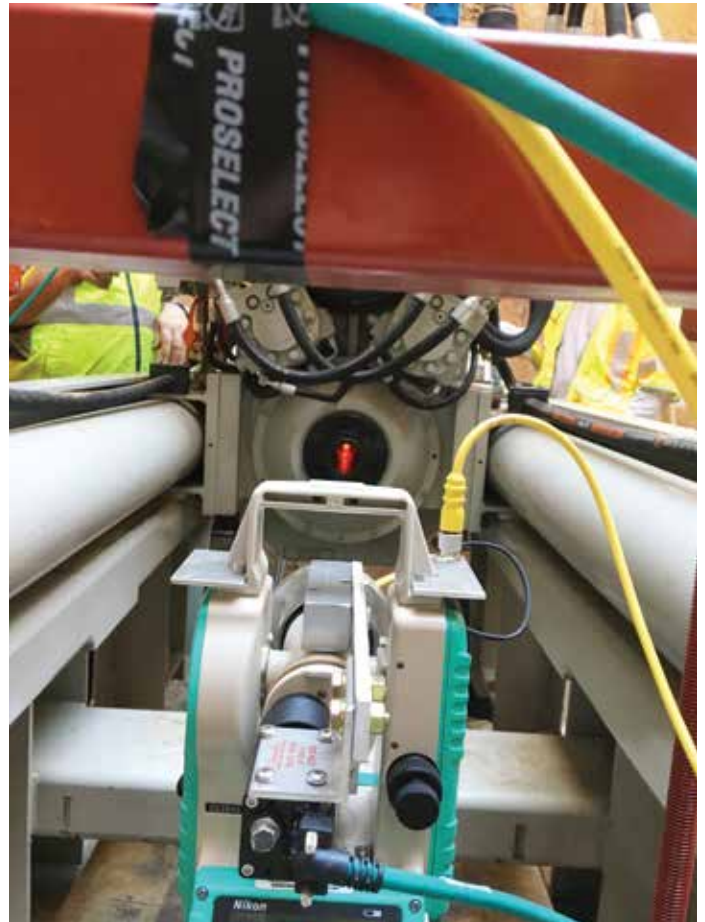
Figure 3. Pilot tube theodolite with integrated camera and visible LED illuminated target
