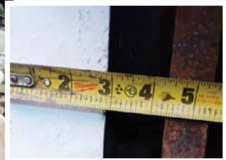
Figure 6. Gusset plates welded to the adapter ring (left); and 1.5-inch gap between the MTBM and the first casing (right)
