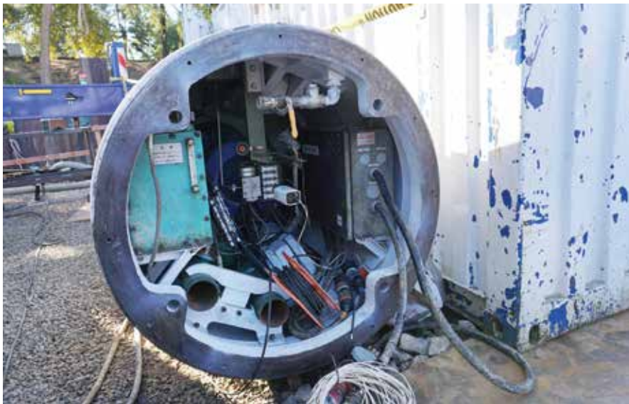
Figure 5. Camera, slurry pipe, water pipe, and target visible in MTBM rear
