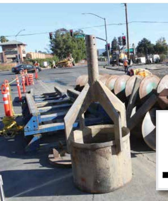
Figure 4. PTGAB reaming head/casing adapter (left) and setup (right)
