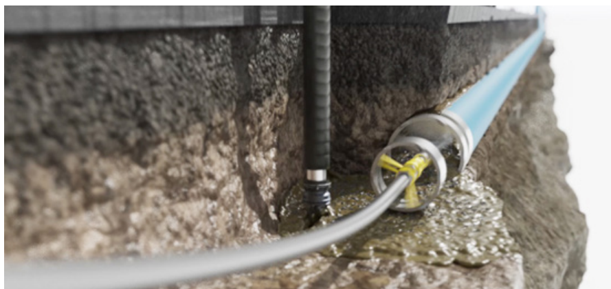
Figure 5. The slurry mix is vacuum excavated from the access pit and hauled away for disposal
