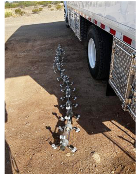
Light train UV-cured the liner at a rate of approximately 3 feet per minute
